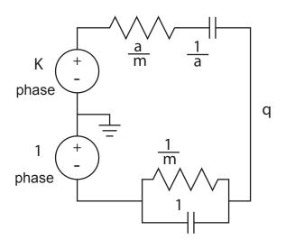
A family of 8 all-pass filters with a from 0.50 to 0.80 achieve ideal opposite sideband performance with m between 1.084M and 1.088M. In the simulator, set the phase of the voltage sources in the q network as a parameter stepped between -90 to +90 degrees. Then plot the output as V(i) + V(g).
